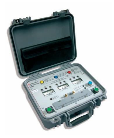
The unique failsafe design of the SD300 incorporates a two-handed push button operation to initiate and maintain the energy discharge, ensuring that the operator cannot come into contact with the live circuit. In addition, the operator is totally isolated from the discharged energy by a fully insulated and robust instrument case rated at IP66.
